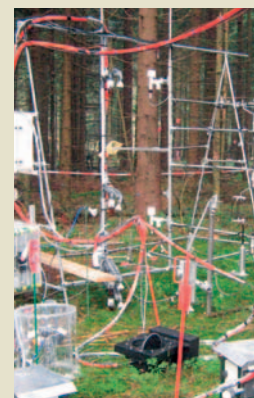
Middle: At the interface 'forest canopy/atmosphere': Micrometeorological instrumentation at the main EGER tower for the measurement of fluxes of non-reactive and reactive trace gases by aerodynamic gradient and eddy covariance techniques.
