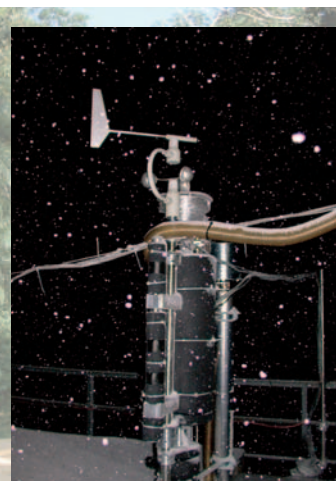
Counterflow virtual impactor inlet system at the Jungfrauoch research site.
