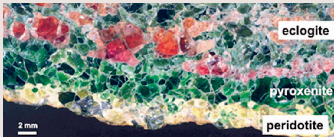
Recycled former ocean crust is converted to (red garnet-bearing) eclogite by high pressure in the mantle. When eclogite melts, it reacts with normal mantle peridotite and forms a new rock consisting of the single mineral, dark green pyroxene.
